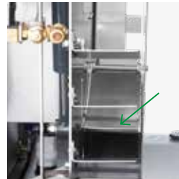
Angle sensor & hydraulically adjustable flaps (for HQS)
